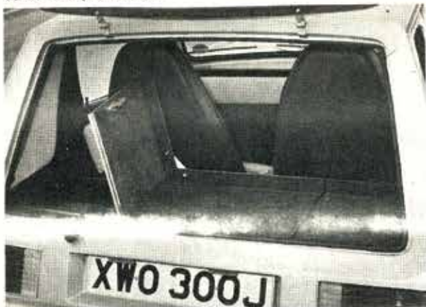
REAR "luggage tray" behind seats is reached through open tail-gate, and covers the "battery store" below. Driver has cockpit gauge to advise when power is low.
