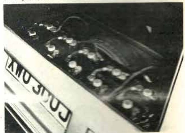
AT PRESENT, heavy lead-acid batteries with low performance and short life are used, but Leyland's Electricar team says a breakthrough on a high-output zinc-air battery is imminent.
